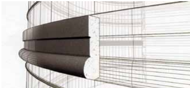
Three-dimensional CADD models were used to study the profile of curved panels at the 390 Interlocken Crescent project in Broomfield, Colo. These drawings then were converted to shop drawings.
