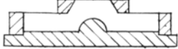
C: INVERTED ARRISE Additional formwork plus additional labor to daily remove and replace back pans.
