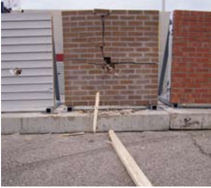
Test two shot the 2 x 4 through a brick wall with wood frame. Surprisingly, it's not all that much safer than siding. What you don't see are the pieces of brick that went flying through the back side of the panel. This wall introduced even more projectiles into the house.
