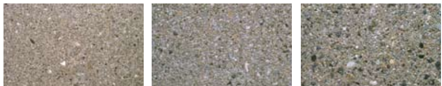
Examples of light, medium, and heavy acid-washed textures.
