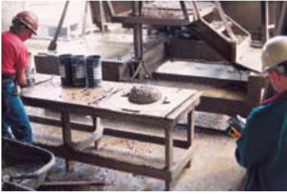
The slump test is a measure of concrete consistency. It is a way to test that the concrete has been made in accordance with design specifications.
