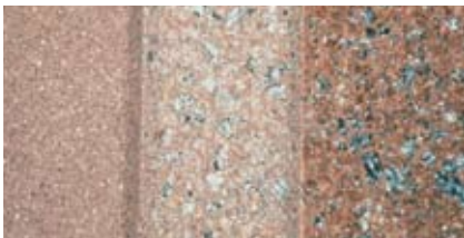
The single concrete mix shown here has three different finishes. From left to right, they are acid etch, sandblast, and retarded. This multiple-finish technique offers an economical, yet effective, way to heighten aesthetic interest.
