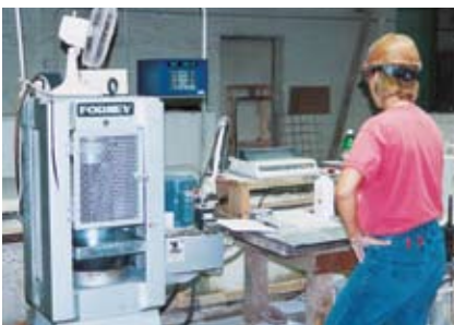
Sample cylinders are loaded and tested to satisfy the specified strength.
