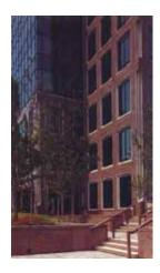
Figure 17 Separate corner pieces are used at BellSouth Campanile in Atlanta to interrupt the wall plane at the corner, emphasizing the corners by vertically articulating the larger multistory lobby space at the base from the typical floors above.
