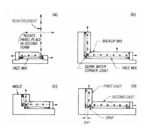
Figure 5 Alternate casting approaches.
