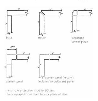
Figure 4 Typical corner and return details.
