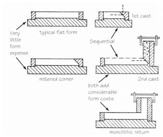
Figure 8 Corner - return molds.
