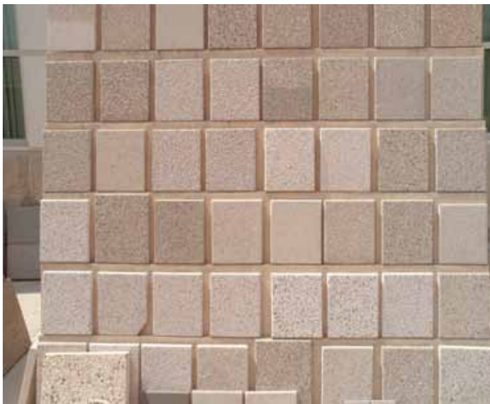
Figure 3 Samples show color, finish, and texture at the precasting plant. (Courtesy Paul Grigonis)
