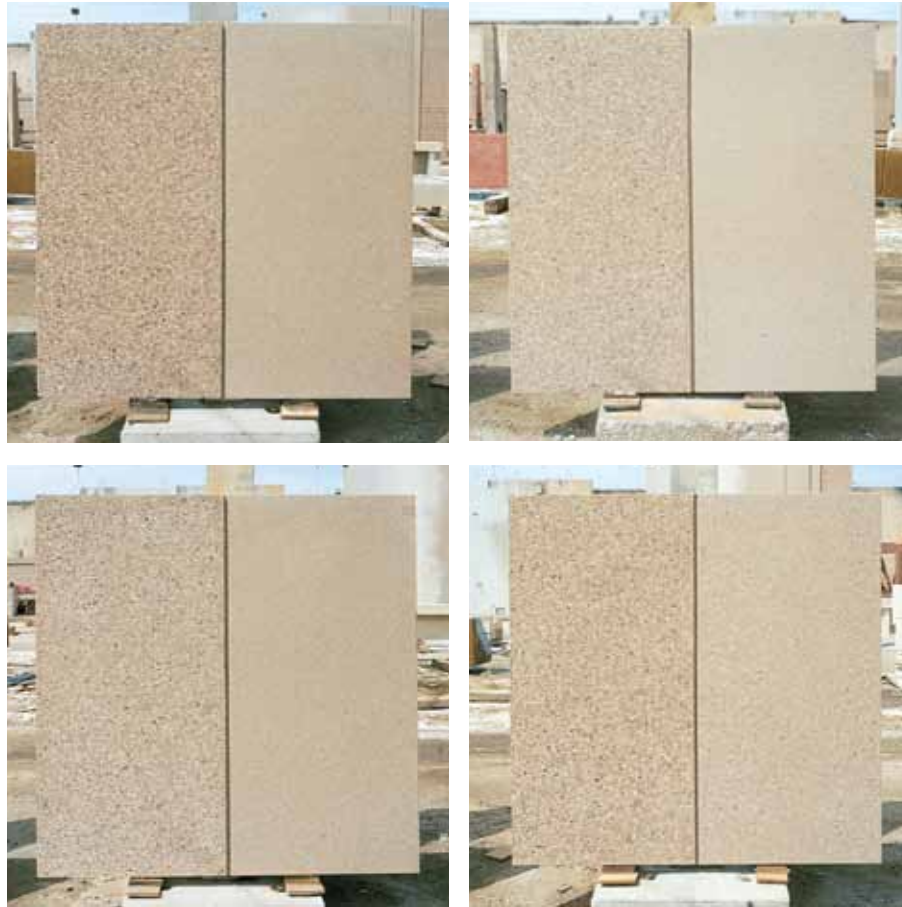
Figure 5 These range samples show retarded finishes on the left and acid-etched finishes on the right.
